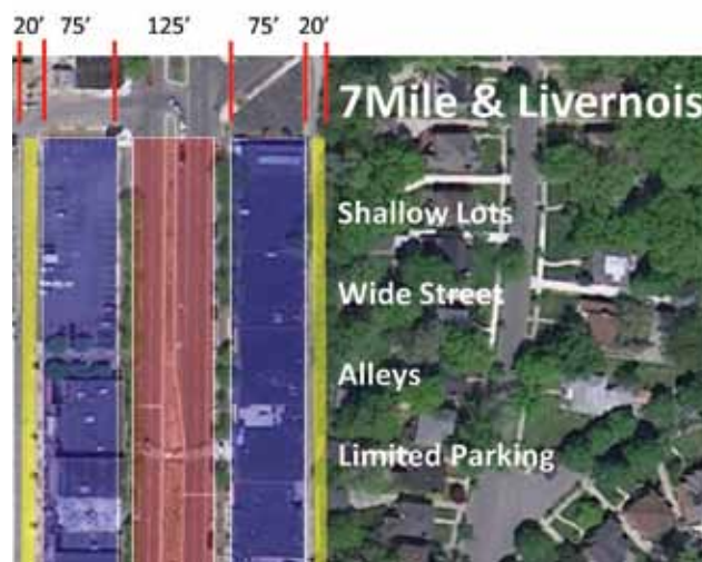
Alleys (shown in yellow) separate Livernois Avenue’s shallow commercial lots from the residential neighborhood.
